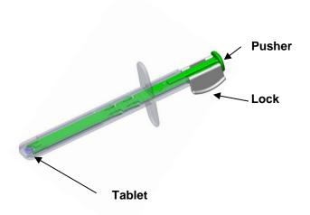
2. Remove the white Lock from the green Pusher by squeezing the sides together and detaching from Pusher. Discard the Lock.
